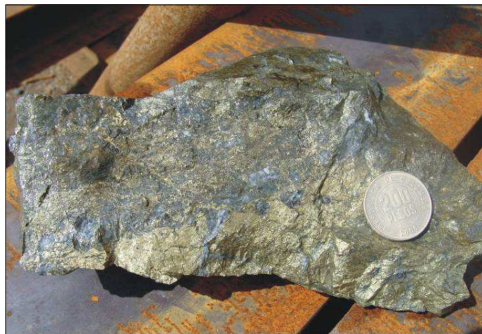
Figure10. Photo of pyrite-chalcopyrite massive sulfide from the El Roble mine, Colombia.
